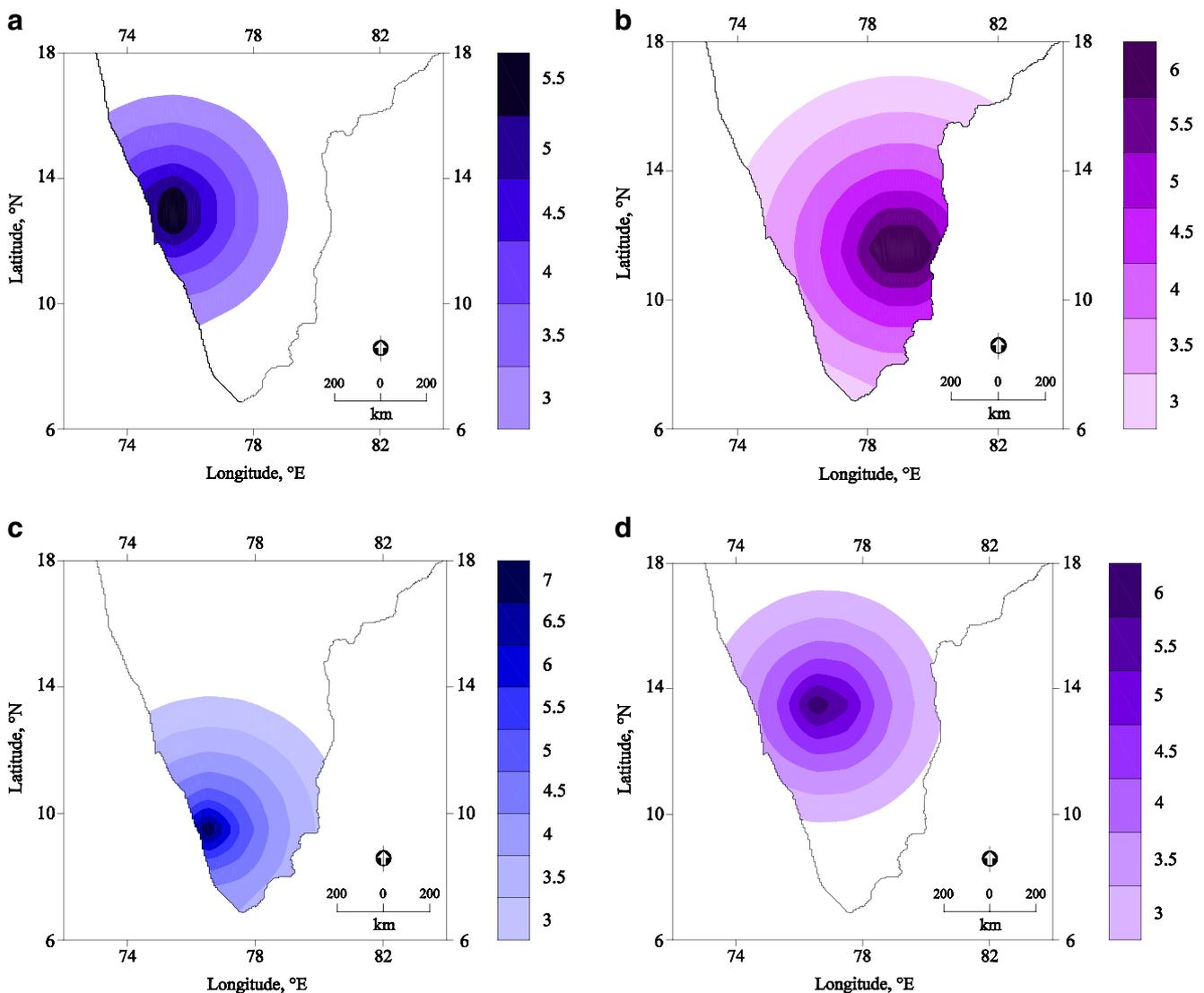
**Fig. 2** a Expected intensity due to probable source zone 1 (Z-1) with maximum magnitude of  $M_w$  5.8. b Expected intensity due to probable source zone 2 (Z-2) with maximum magnitude of  $M_w$  6.4. c Expected Intensity due to probable source zone 3 (Z-3) with maximum magnitude of  $M_w$  6.0. d Expected intensity due to probable source zone 4 (Z-4) with maximum magnitude of  $M_w$  5.8. e Expected intensity due to probable
