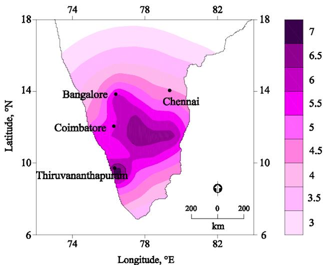
**Fig. 3** Expected maximum intensity due to occurrence of earthquake in the any of the probable source zones
